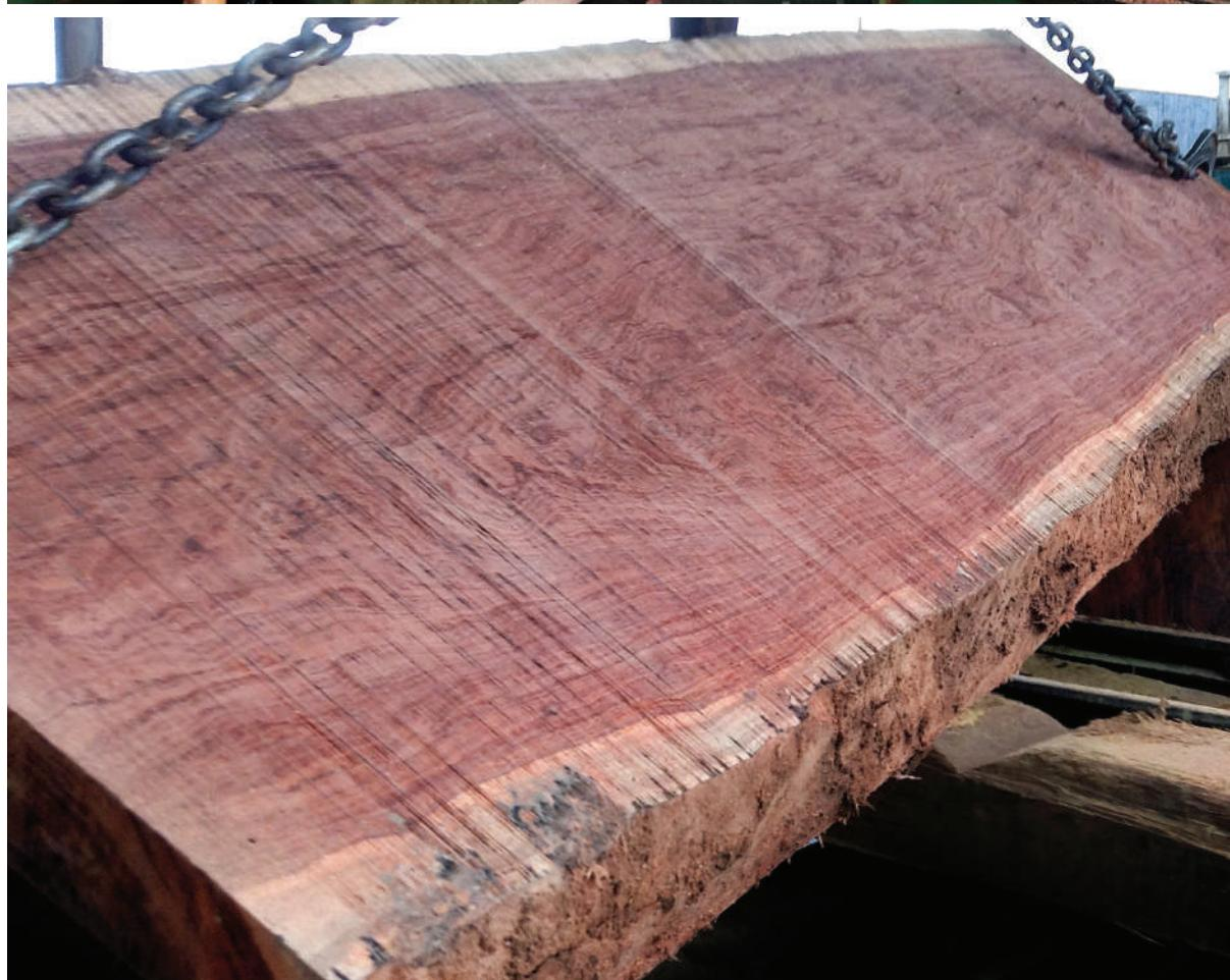
The giant logs are carried by special lifting equipment and placed on a leveled carriage prior to sawing.
