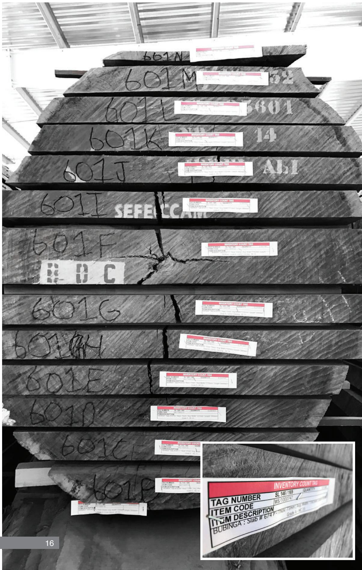
Once dry, slabs are packed back into the original log configuration, forming what is referred to as a boule.
